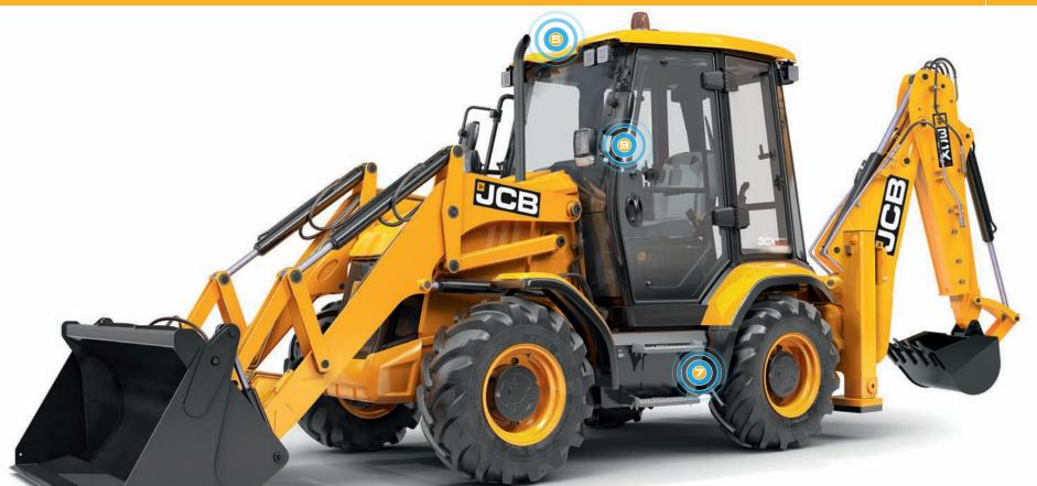
**Z** Twin anti slip steps with an open grille design prevents build up of material for safe entry/exit to machine.
