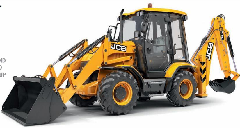
A 3-in-1 machine, the 3CX Compact can be a compact excavator and wheel loader, with skid steer attachment versatility.
