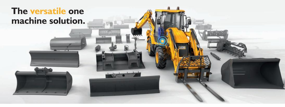
The 3CX Compact is not only designed for the vast range of tool carrier attachments. It also has the ability to pick up a wide range of skid steer loader attachments. Bi-directional pipework and a handheld tool circuit provide even greater versatility.
