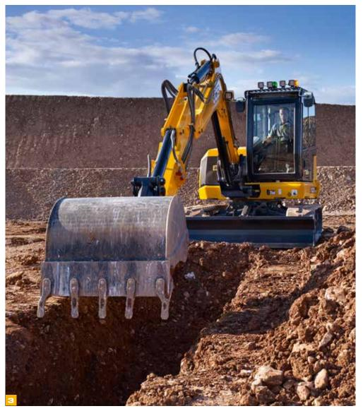
The fully compliant ROPS and TOPS\* cab has excellent front visibility courtesy of a 70/30 front screen split. It also provides a clear view of the front right track for easy, safe trench digging and manoeuvring. Overall, we have improved overhead visibility from the cab making truck loading easier and safer.
